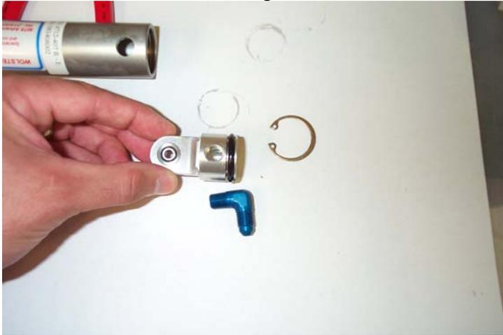
Grease the O-ring using Mil-H-5606 hydraulic fluid, Lubriplate No. 105, or similar.
