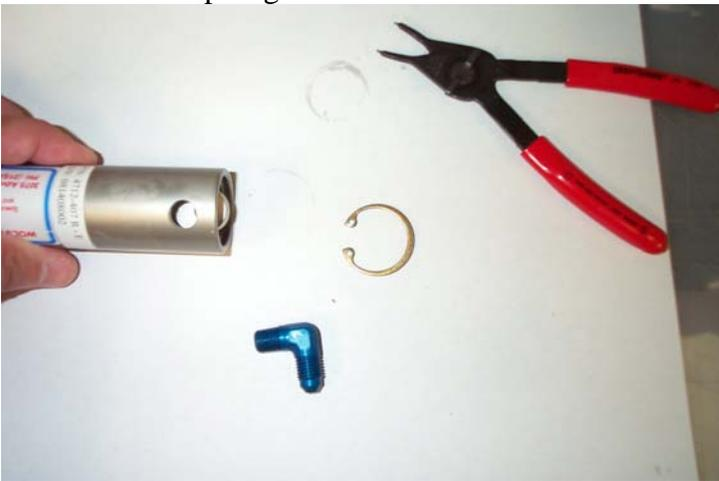
Pull the actuator end out of the cylinder.
