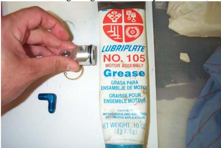
Slide the actuator end into the cylinder without cutting or nicking the O-ring.
