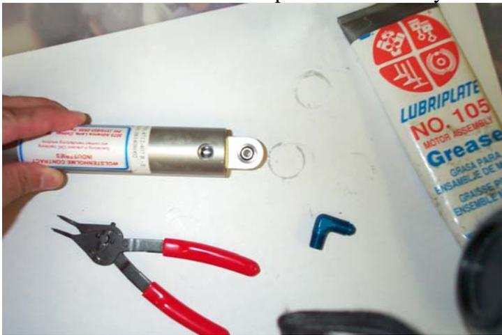
Coat the 90 degree fitting threads with thread compound (Loctite™ 565) then reinstall the fitting to approximately the angle shown.
