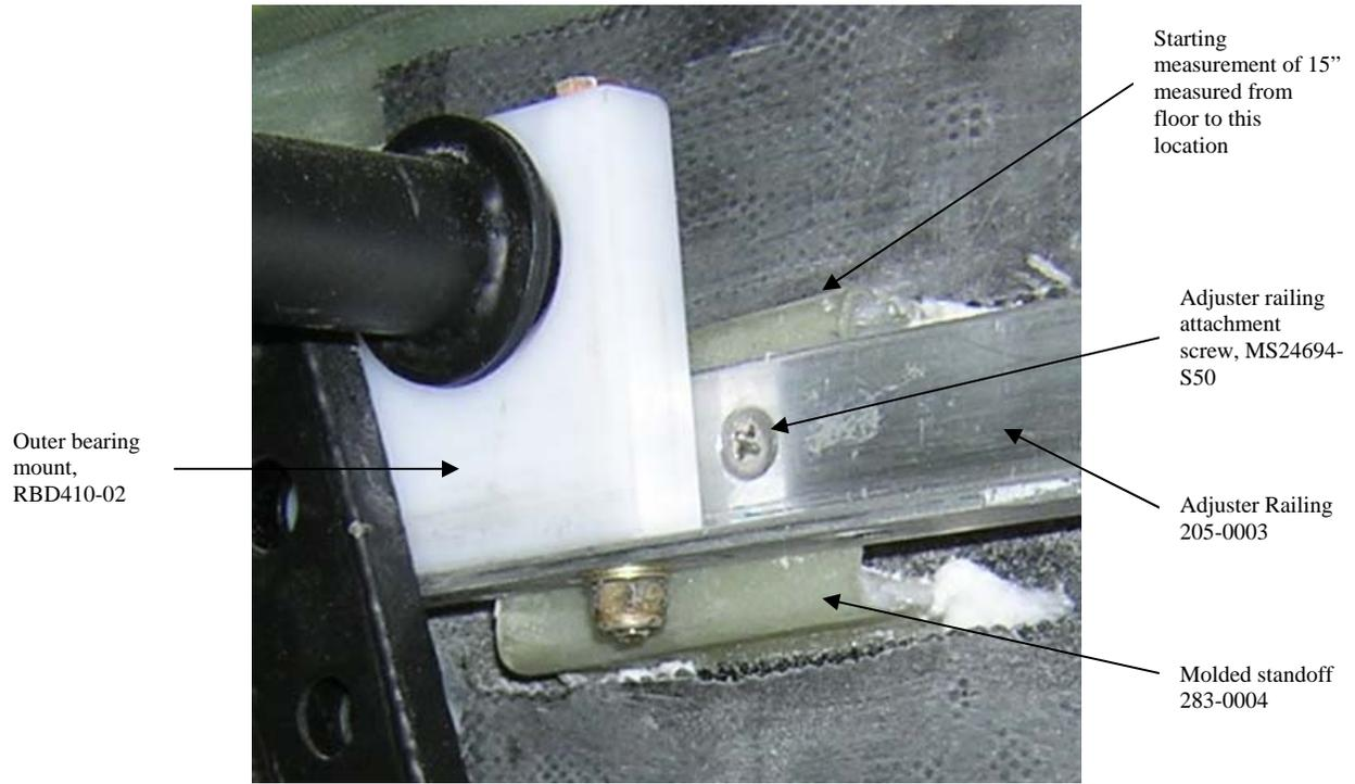
**Figure 12.3.E.4 Railing attached to Firewall**
