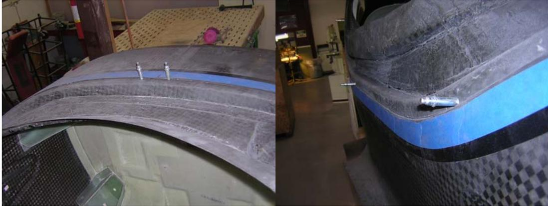
When fitting the stiffener use 3/32" clecos to hold it in place, it makes a smaller hole and is easier to work with. Only use the amount needed to hold the stiffener from moving as you work, it is unnecessary to put them every 2-3 inch's in this stage.
