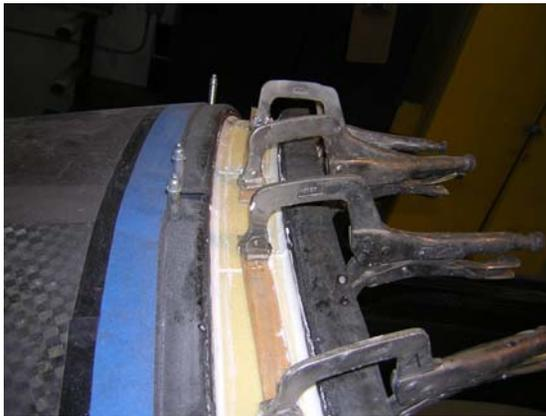
Before fitting the stiffener you need to place 1/8-inch shims around the top of the door seal joggle approximately every 12-14-inch's. You want the stiffener to rest on the shims as best as possible. The stiffener may bind on some of the shim's (**this is not a problem**) just remove the shim and keep fitting the stiffener the best you can, it will not be perfect.
