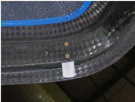
The best time to put in your canopy alignment pins and the latch striker plates would be after the hinge is installed and before you bond the skin on. You may even like to do it before you bond the windshield on so that you don't have that extra weight.
