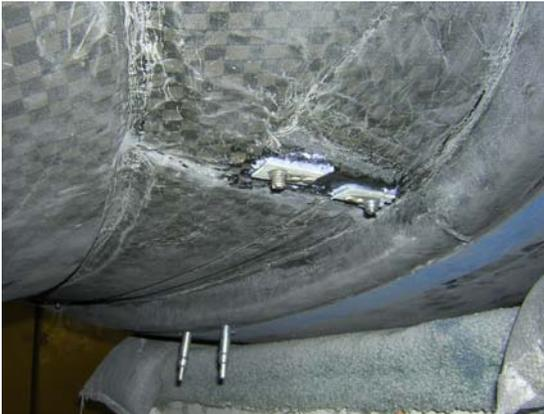
When you are aligning the canopy hinge you need to make sure that you have your 1/8" spacer underneath the hinge. You will need to do some grinding on the spacer so that it will sit flush on the canopy stiffener. To align the hinges with each other, bolt the canopy hinge support to the hinges. To align the hinge with the firewall use a 6" scale and measure off the core to a stationary point around the bearing on the hinge, you will need an even measurement on both sides of the hinge to make it
