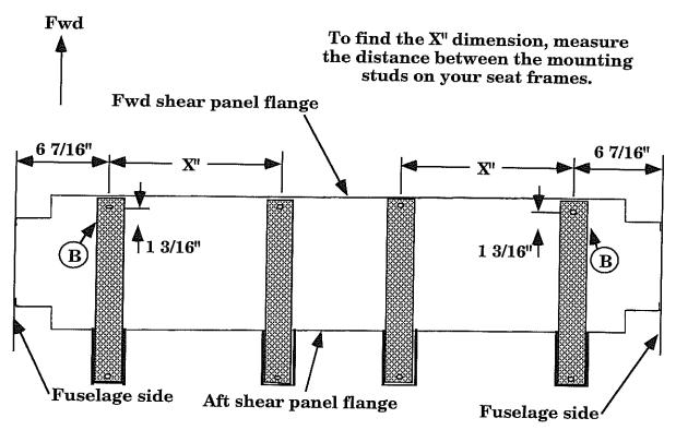
NOTE: The outbd, fwd mounting holes (B) of each seat will also be used to attach the jack point. These two holes should be drilled 1 3/16" from the aft face of the fwd shear panel. If you have already installed the jack point weldments, these holes will, of course, already have been drilled.
