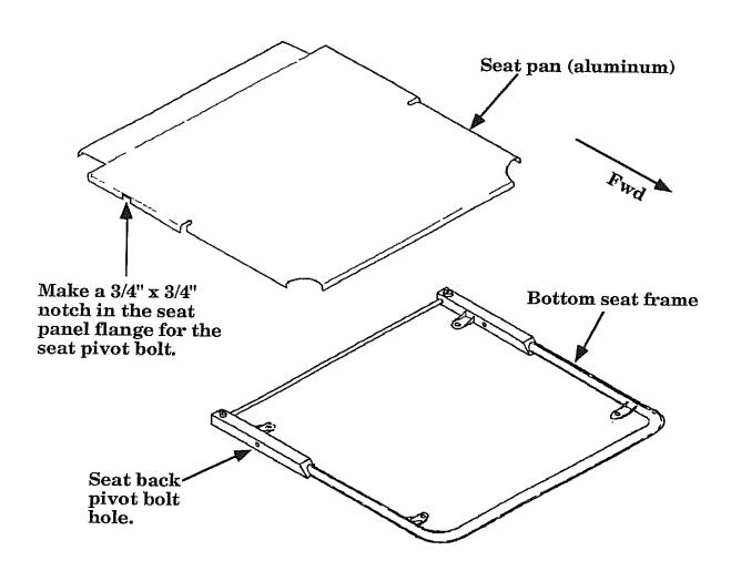
A1. Place the aluminum seat pan onto the bottom seat frame. Make a 3/4" wide, 3/4" high notch in both sides of the aluminum pan, centered on the seat back pivot bolt hole, as shown in Figure 25:A:1.
