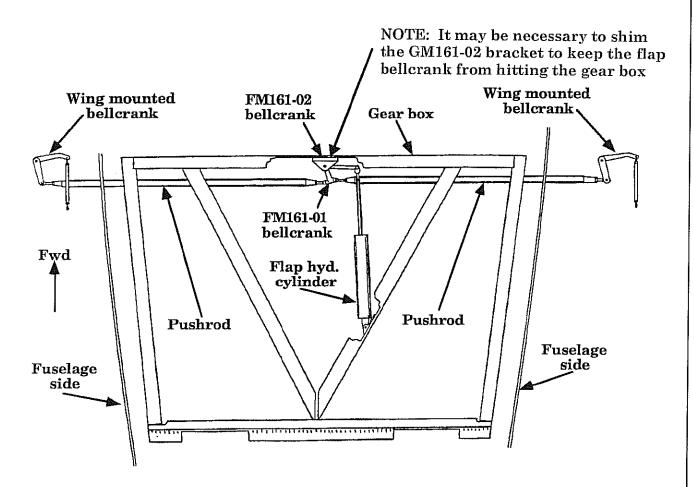
NOTE: Be sure you have the proper hydraulic cylinder (HC-09). The stroke of this cylinder was shortened from the earlier version (HC-08) so a secondary stop would not be necessary.
