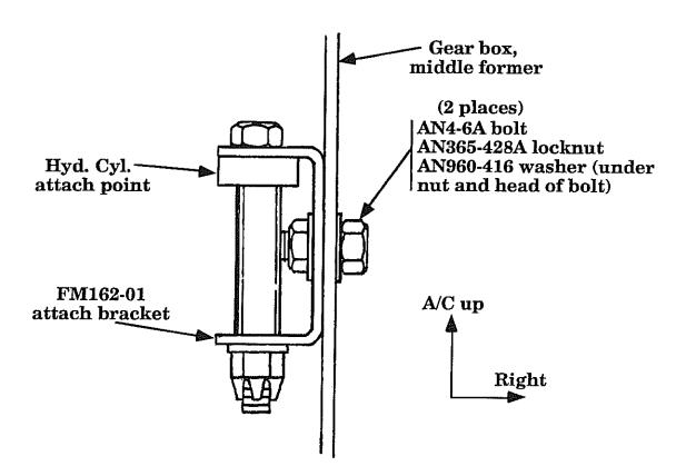
NOTE: It may be necessary to remove FM162-01 bracket in order to install the bolt point down.
