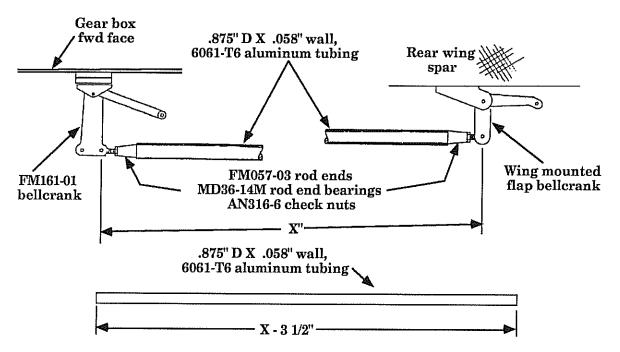
\* NOTE: Right pushrod is shown, Make left pushrod the same way. Also notice that the FM161-01 bellcrank and the inbd wing bellcrank are both in the "trail" position, parallel with the line of flight.
