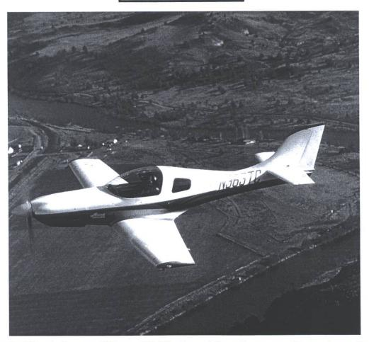
Lancair's 360 turbo has over 150 hours of flight testing and the performance numbers are impressive. The engine has a critical altitude of 18,000 ft. and maintains 75% power through 24,000 ft. Cruising at 27" manifold, 2200 RPM and 10.5 gph, the airplane trues out at 230 kts. at 18,000 ft and 240 kts. at 24,000 ft.
